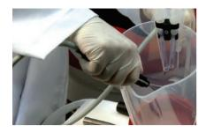
Reattach the bottle to the unit, and run the pink solution through all the dental chair instrument lines until the pink solution comes out visibly and all the solution from the bottle is used up. Do not forget about running the solution via the spittoon. Make sure all lines are now completely filled with the pink solution. The tubes should feel very warm. Now all the lines are internally covered with the BRS® PRECLEANER.
