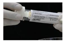
Just before use turn the dip slide counterclockwise and remove it from the tube.
