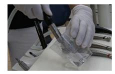
Fill a cup with a mixture of water coming from all the water lines (turbines, contraangles, handpieces, scalers, triplex syringes an spittoon)
